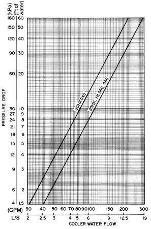
Fig. 16 — Cooler and Condenser Water Pressure Drop
